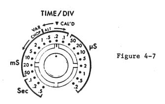
The CALIB voltage signal is a square wave of approximately 1 kHz. When the TIME/DIV knob is set in the 0.2 mS/DIV position, one cycle of the square wave is displayed with a horizontal magnitude of approximately 5 DIV.
