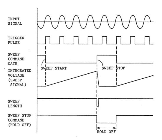
Figure 6-11. A timing chart of the sweep circuit
