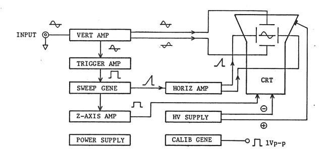
Figure 6-1. A block diagram of the oscilloscope
