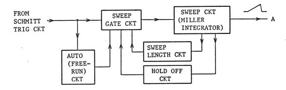
Figure 6-10. A block diagram of the sweep generator circuit
