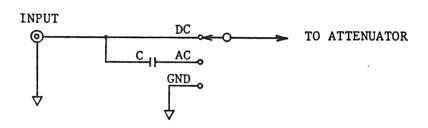
Figure 6-3. The input circuit
