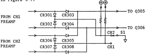
Figure 6-7. The CH1/CH2 selector circuit
