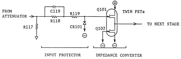
Figure 6-5. The input protector and impedance converter
