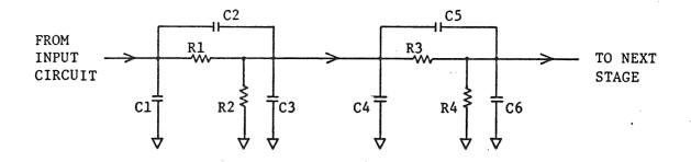
Figure 6-4. An example of combination of attenuator circuits
