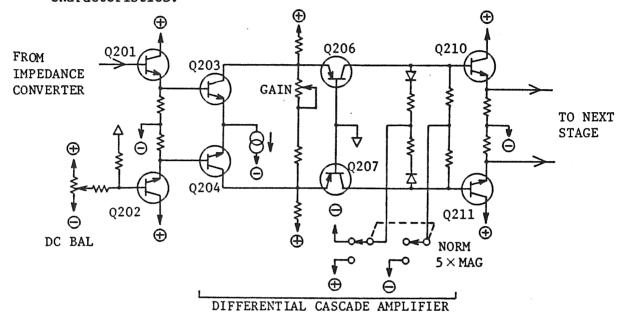
Figure 6-6. The preamplifier (front stages)
