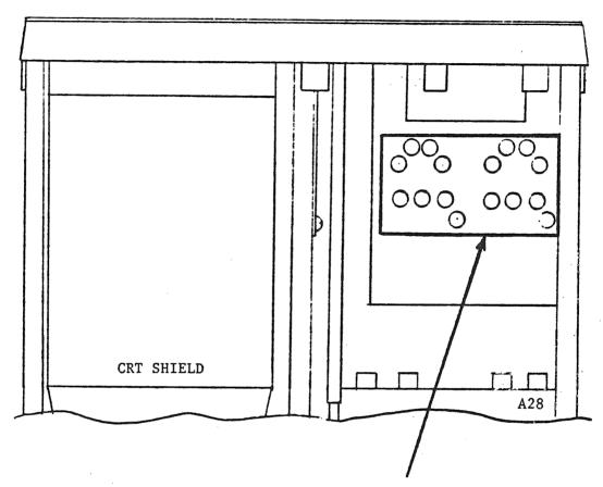
Controls of input capacitances of respective ranges of vertical VOLTS/DIV switches of CH1 and CH2.
