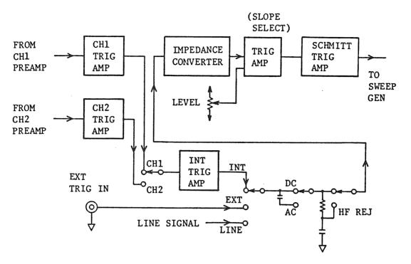
Figure 6-8. A block diagram of the trigger circuit
