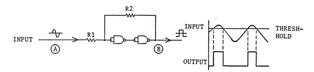
Figure 6-9. Schmitt trigger circuit
