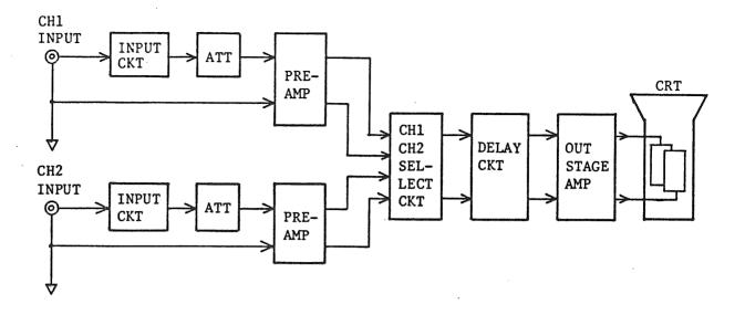
Figure 6-2. A block diagram of the vertical amplifier
