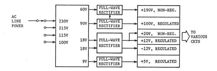
Figure 6-14. The power supply circuit
